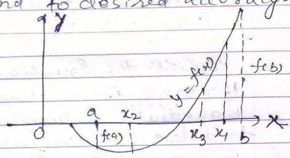
In the adjoining figure  $f(x_1)$  is (+)ve so that the root lies between 'a' and 'x1'. Then second approximation to the root is:
