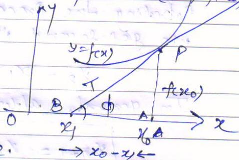
The intercept  $OQ$  on the  $x$ -axis of the tangent to the curve at the point  $P$ , if it is taken as the first approximation
