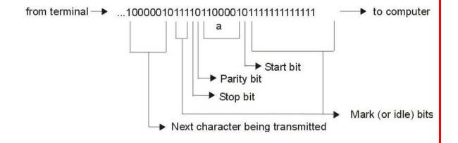
When the mark state is interrupted by a positive voltage (a binary 0), the receiving system knows that data characters are going to follow. It is for this reason that the start bit, which precedes the data character, is always a space bit (binary 0) and that the stop bit, which signals the end of a character, is always a mark bit (binary 1).
