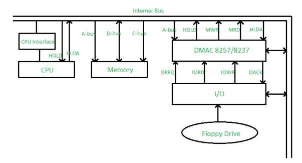
Suppose a floppy drive which is connected at input-output port wants to transfer data to memory, the following steps are performed:
