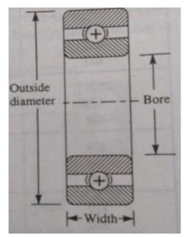
dimensions are a function of the bearing bore and the series of bearing. The standard dimensions are given in millimetres. There is no standard for the size and number of steel balls. The bearings are designated by a number. In general, the number consists of atleast three digits. Additional digits or letters are used to indicate special features e.g. deep groove, filling notch etc.
