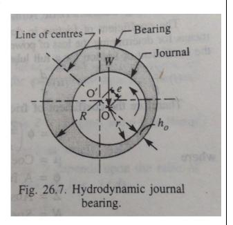
Note: The diametral clearance (c) in a bearing should be small enough to produce the necessary velocity gradient, so that the pressure built up will support the load. Also the small clearance has the advantage of decreasing side leakage. A commonly used clearance in industrial machines is 0.025 mm per cm of journal diameter.
