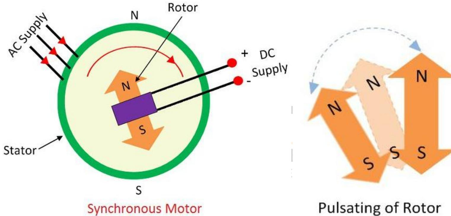
The rotor attracts towards the pole of the stator for the first half cycle of the supply and repulse for the second half cycle. Thus the rotor becomes pulsated only at one place. This is the reason because of which the synchronous motor is not self-starting.
