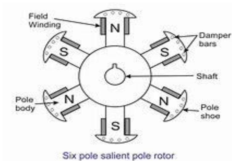
Since the rotor is subjected to changing magnetic fields, it is made of steel laminations to reduce eddy current losses. Poles of identical dimensions are assembled by stacking laminations to the required length. A salient pole synchronous machine has a non-uniform air gap. The air gap is minimized under the pole centres and it is maximum in between the poles.
