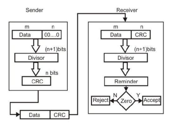
If a k bit message is to be transmitted, the transmitter generates an r-bit sequence, known as Frame Check Sequence (FCS) so that the (k+r) bits are actually being transmitted. Now this r-bit FCS is generated by dividing the original number, appended by r zeros, by a predetermined number. This number, which is (r+1) bit in length, can also be considered as the coefficients of a polynomial, called Generator Polynomial. The remainder of this division
