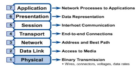
**Layer 1: Physical** - This is the level of the actual hardware. It defines the physical characteristics of the network such as connections, voltage levels and timing.
