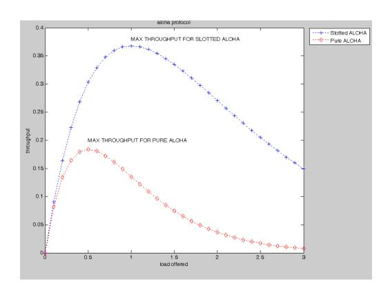
**Result:** Efficiency of Pure and slotted ALOHA is successfully plotted.
