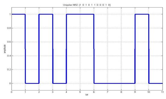
**RESULT** –Unipolar NRZ signal is generated successfully.
